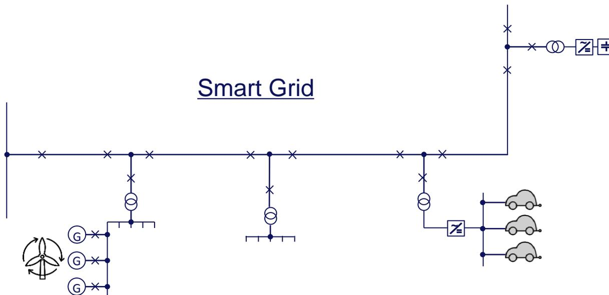
By using a full range circuit breaker feeding a transformer, there is a suitable apparatus to use for disconnection in both fault cases. The protection relay take care of transformer fault in a traditional way.
